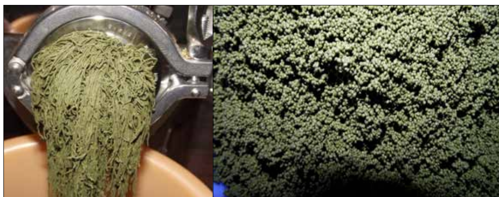
Cold extrusion cum Spheronization (Micro extruded marumerized feed production)
